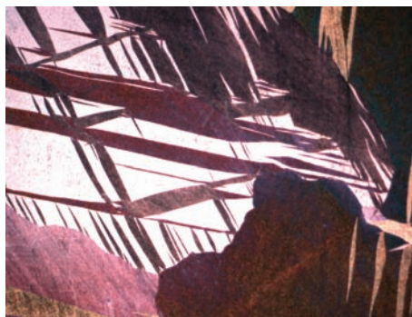
Tin with deformation twins, 1:100
